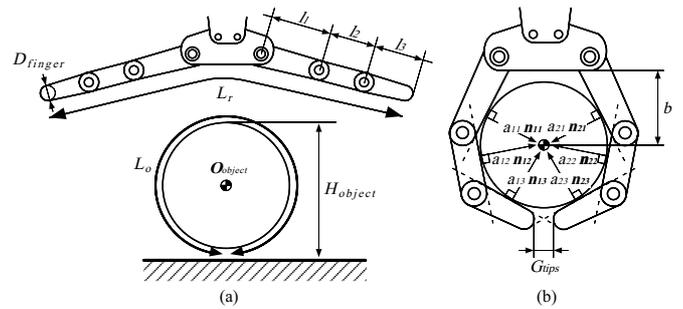
Fig. 7. The relation between the robot hand and the object.
