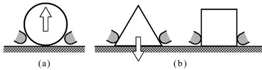
Fig. 15. Examples of objects where the upward force is expected (a) and is not expected (b) by a simple pushing motion.
