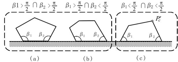
Fig. 18. Grouping of column objects whose cross sections are convex.
