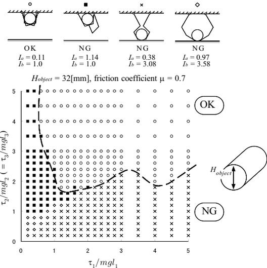
Fig. 11. Success map for a cylindrical object ( $\mu = 0.7$ ).
