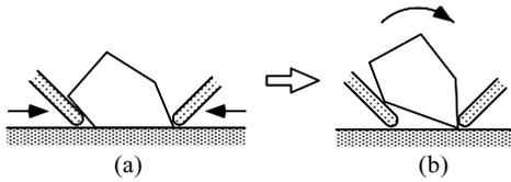
Fig. 19. The wedge-effect at one edge of the object.
